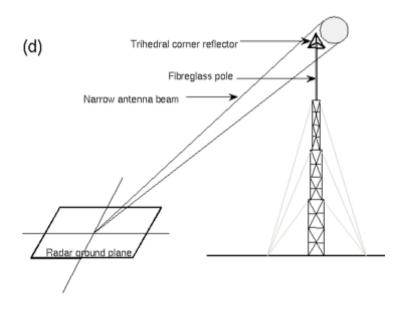
Figure 9. Calibration target.
