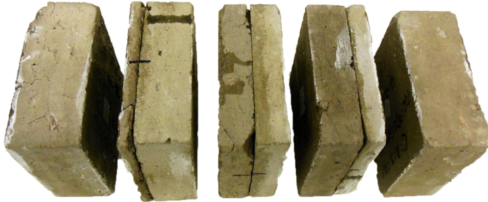
Fig. 2 Concrete specimen samples. From left to right: completely damaged sample, partially damaged sample, half damaged sample, mostly damaged sample, undamaged sample.
