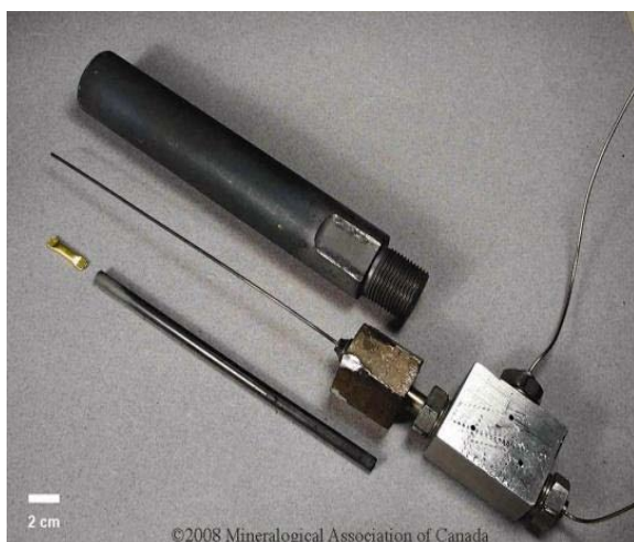
Figure 4. Cold seal reaction vessel, disassembled (800 °C, 2.5 kbar max.; from London 2008, Figure 14-1a).
