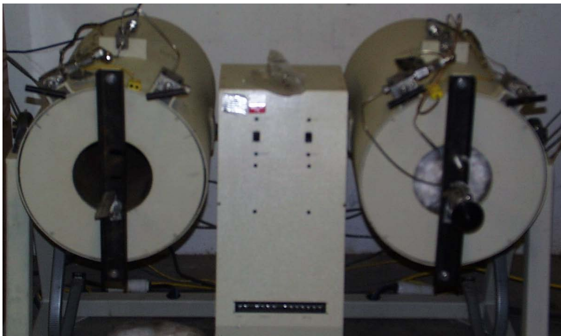
Figure 3. 400 °C /600 bar rocking autoclave rack (autoclave drums are ~24” tall)
