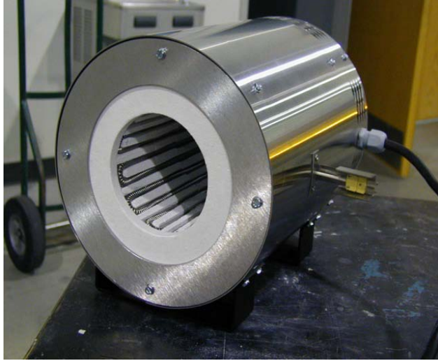
Figure 5. Furnace assembly for cold seal apparatus
