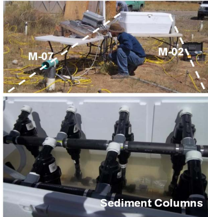
Figure 3. Recirculation experiment showing the injection well (M-02) and the extraction well (M-07). On the left table in the upper photo are pump and flow controls. On the right table is the “cooler” that was modified to serve as a constant head reservoir for reinjection into M-02. Not shown is the metering pump that was used to deliver urea and molasses into the water pumped from M-07. The cooler also served as a constant temperature bath (lower photo) for sediment columns that were subjected to advecting groundwater and served as analogs for injection well aquifer sediments (“active” sediments).
