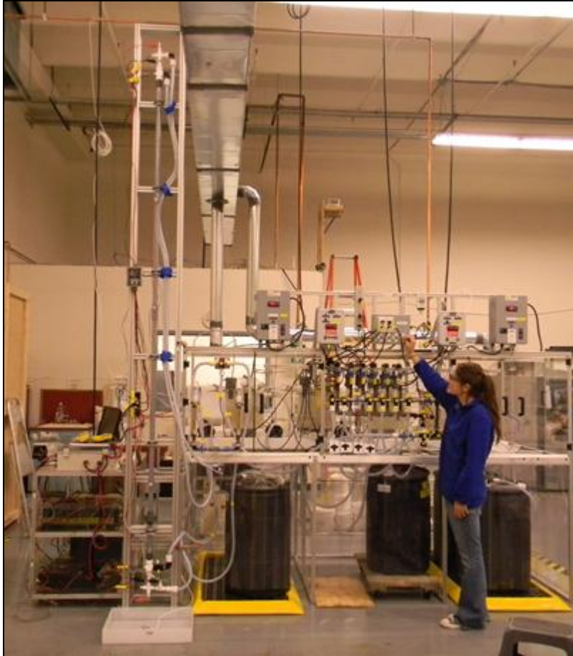
Figure 5. Photograph of apparatus for plating catalyst coatings on ID and OD surfaces of 10' long membrane tubes.
