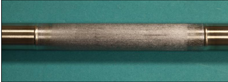
Figure 6. Tubular hydrogen membrane with a stainless steel stub welded to each end.
