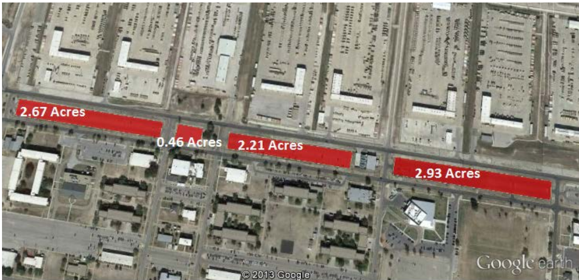
Figure 6. Aerial view of the areas evaluated for PV carports (comprises only a small section of the space available for carports at the MC)
