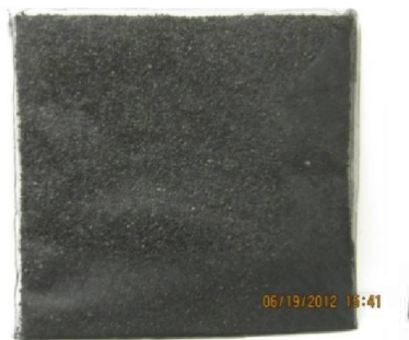
Figure 3: Filter element 2b, a pad filter containing activated carbon.
