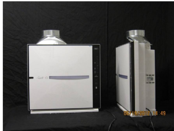
Figure 5: Photographs of the modified air cleaner. The sheet metal fitting at the top is a temporary feature installed to facilitate sampling from the outlet airstream.
