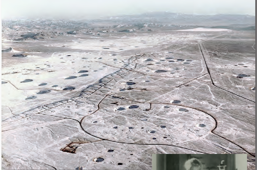
Aerial view of Yucca Flat showing subsidence craters from historical underground nuclear tests.
