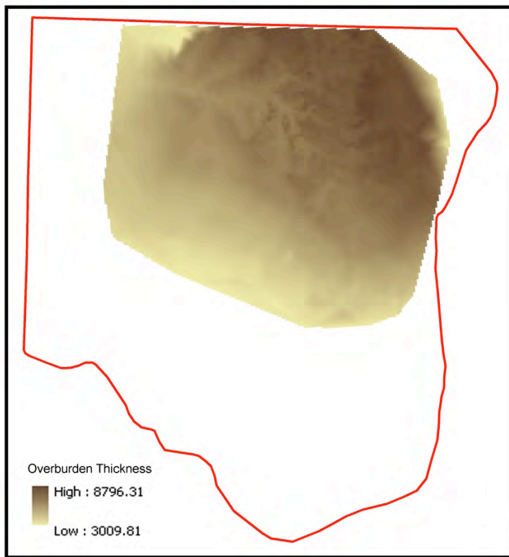
Figure 5.21. A map of the overburden (ft) on top of the Dakota Group.
