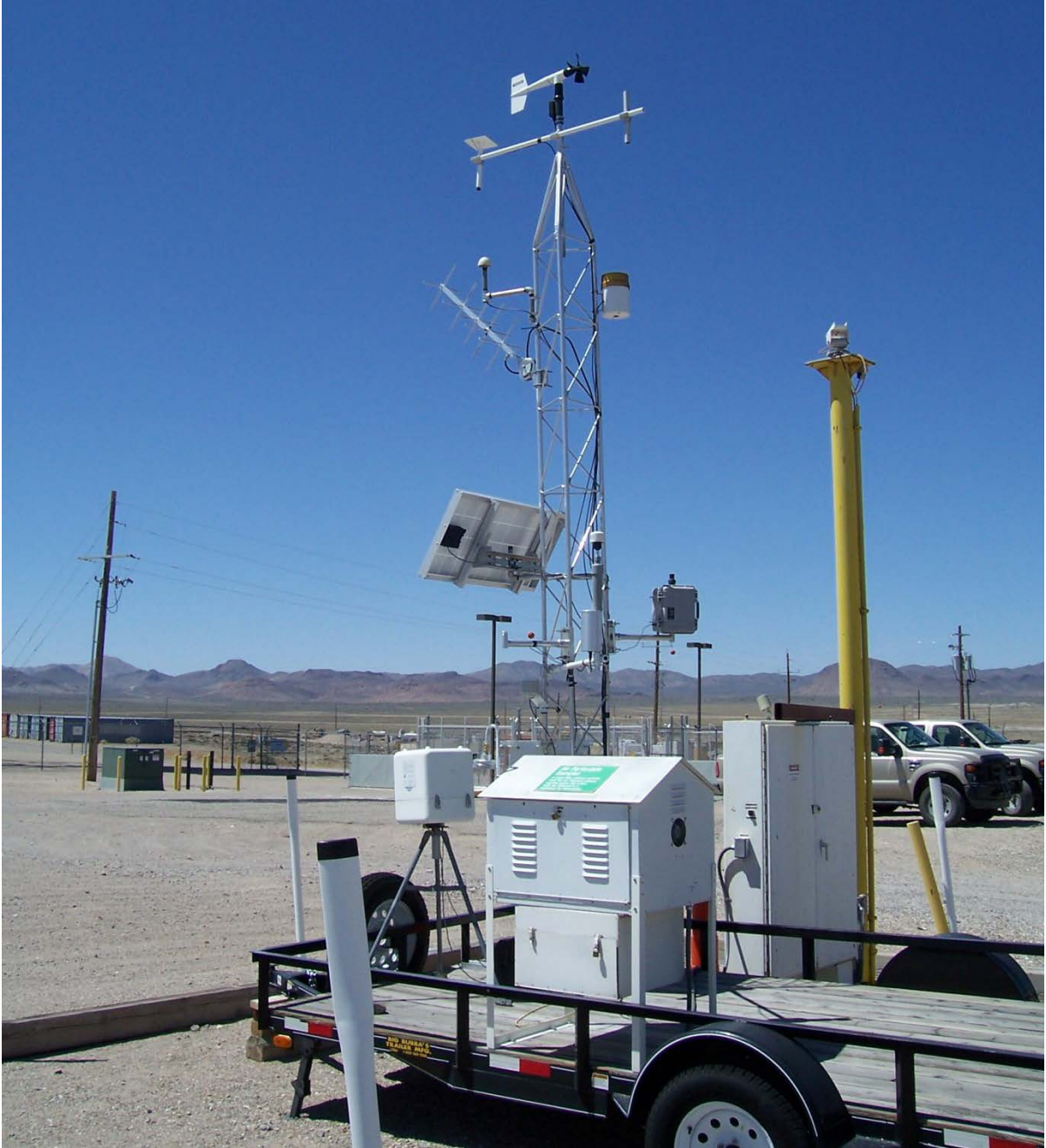
Figure 3. Station 400 is a trailer mounted radiological and meteorological measurement system located near the Range Operations Center (ROC) in the Sandia National Laboratories compound on the Tonopah Test Range.
