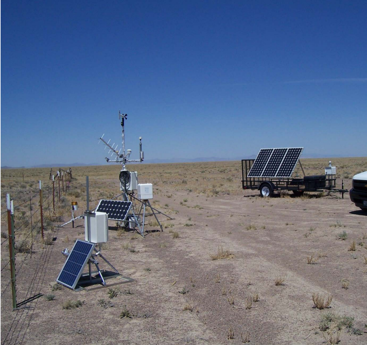
Figure 5. The solar powered air sampler, saltation sensor, and meteorological tower (center right, foreground left, center left, respectively) at Station 402 are located along the north fence that bounds the Clean Slate 1 contamination area.
