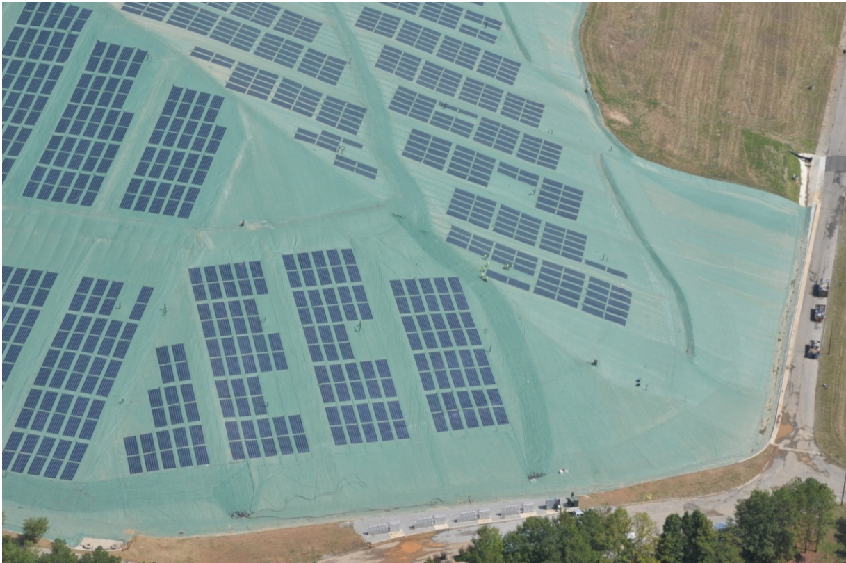
Figure 5-4: Hickory Ridge Road Landfill – Geomembrane solar cover
