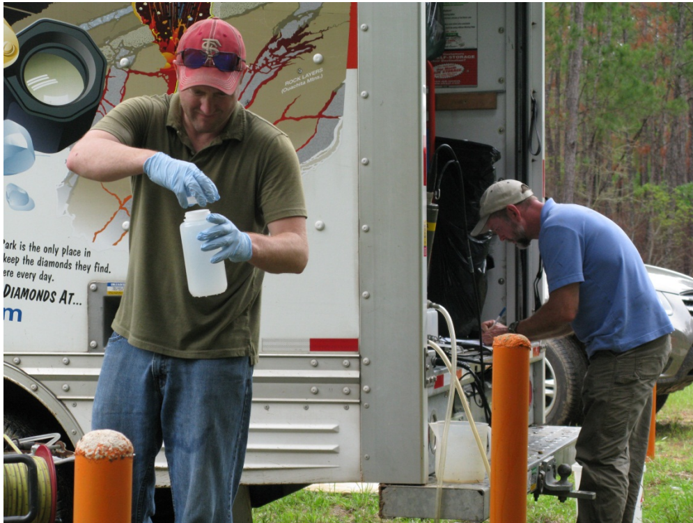
Image A-3. Sealing a sample container of water collected from well HM-3. In the background, the technician is working on sample chain-of-custody paperwork for the analytical laboratory. Clean gloves are worn so as not to contaminate the sample.
