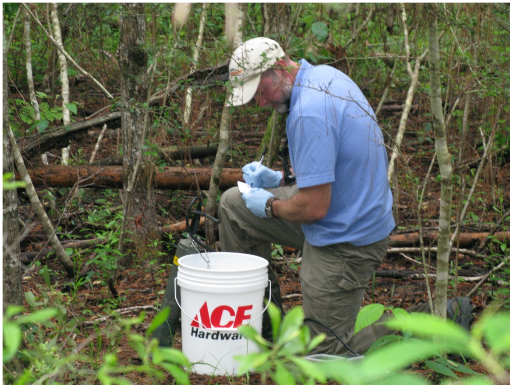
Image A-4. Recording field measurements (pH, specific conductance, and temperature) made on a surface-water sample collected from Half Moon Creek where it enters the site from the south.
