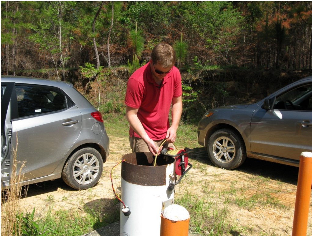
Image A-8. A depth-to-water-level measurement is made in well SA5-4-4.
