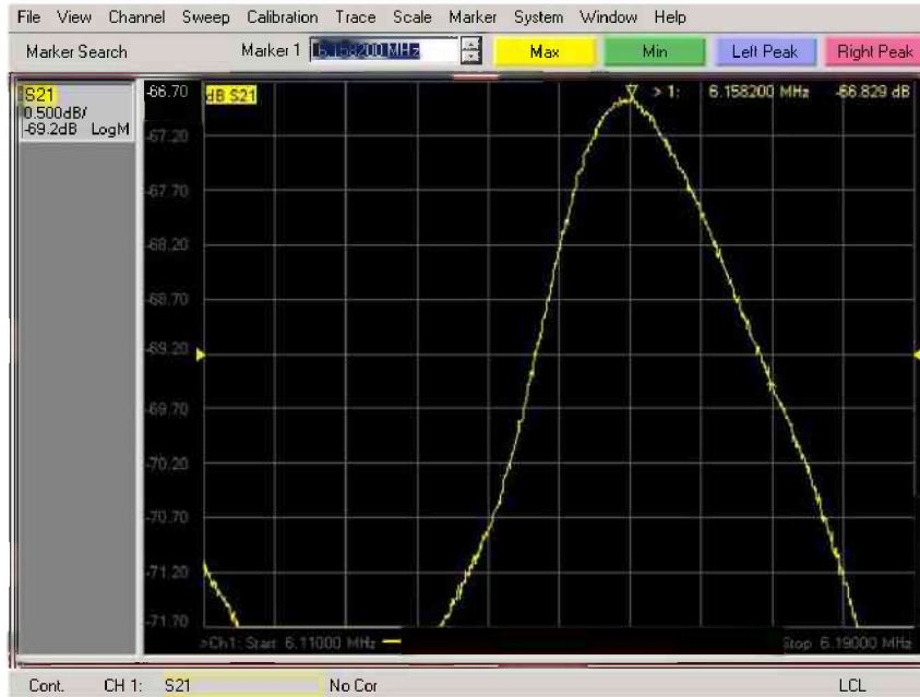
Figure 5. 28 Sensor Response at dry air with 0%RH.
