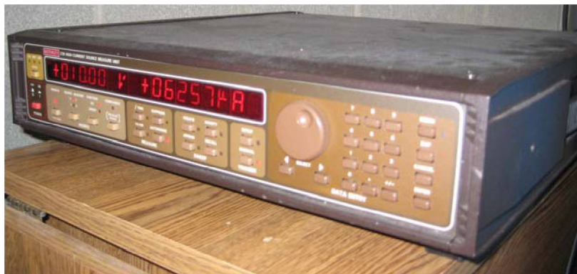
Figure 5. 2 Keithley 238 current source measurement unit.
