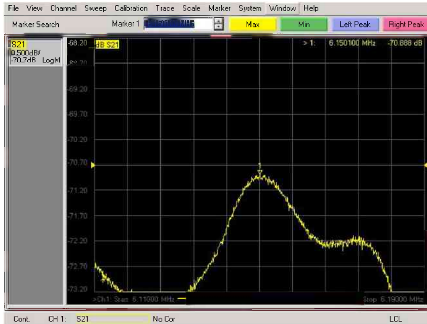
Figure 5. 34 Sensor Response 84.3%RH.
