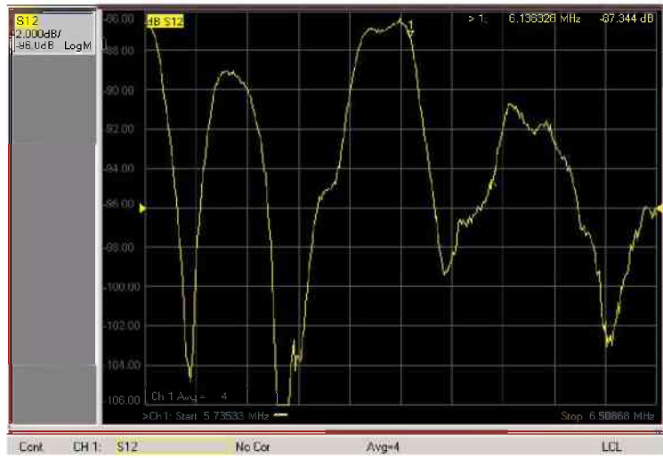
Figure 6. 10 Sensor response with antenna in series configuration at 10mm distance.
