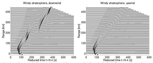
Figure 3, signal recorded at stations with atmospheric wind. Subfigures show downwind of source (left) and upwind of source (right).
