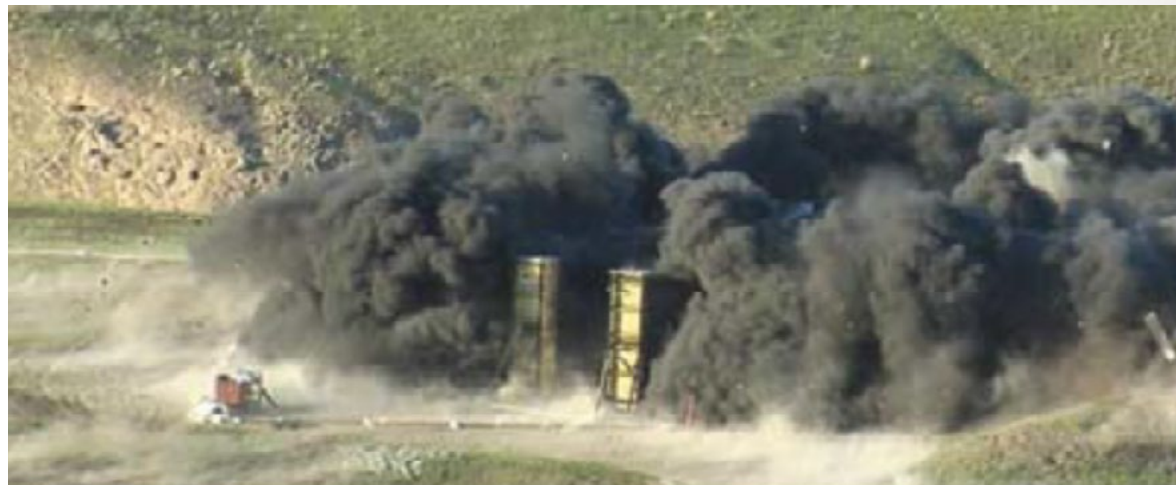
An arena test at the Laboratory's Site 300 used an aeroshell fashioned from commercial carbon composite panels. This experiment validated warhead performance prior to the sled test.
