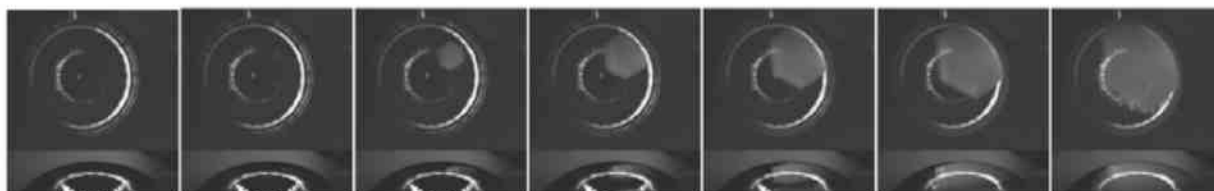
Figure 2.6: Pair of high-speed Photron SA2 cameras allows us to pinpoint nucleation sites and measure the droplet contact angle. In this film strip each frame represents a time step of 2 ms, or every 20th frame at a sample rate of 10 kHz. The nucleation site is evident at the center of the hexagonal crystal when the film is viewed in reverse.
