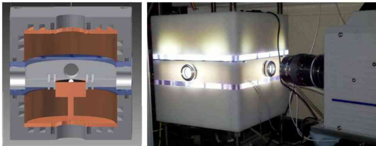
Figure 2.5: The left panel is a half cut schematic of the nucleation chamber. The test droplet is depicted as a white hemisphere resting on the dark silicon substrate. The right panel is an image of the actual chamber with a Photron SA2 camera arranged for horizontal imaging of a droplet in the middle of the chamber.
