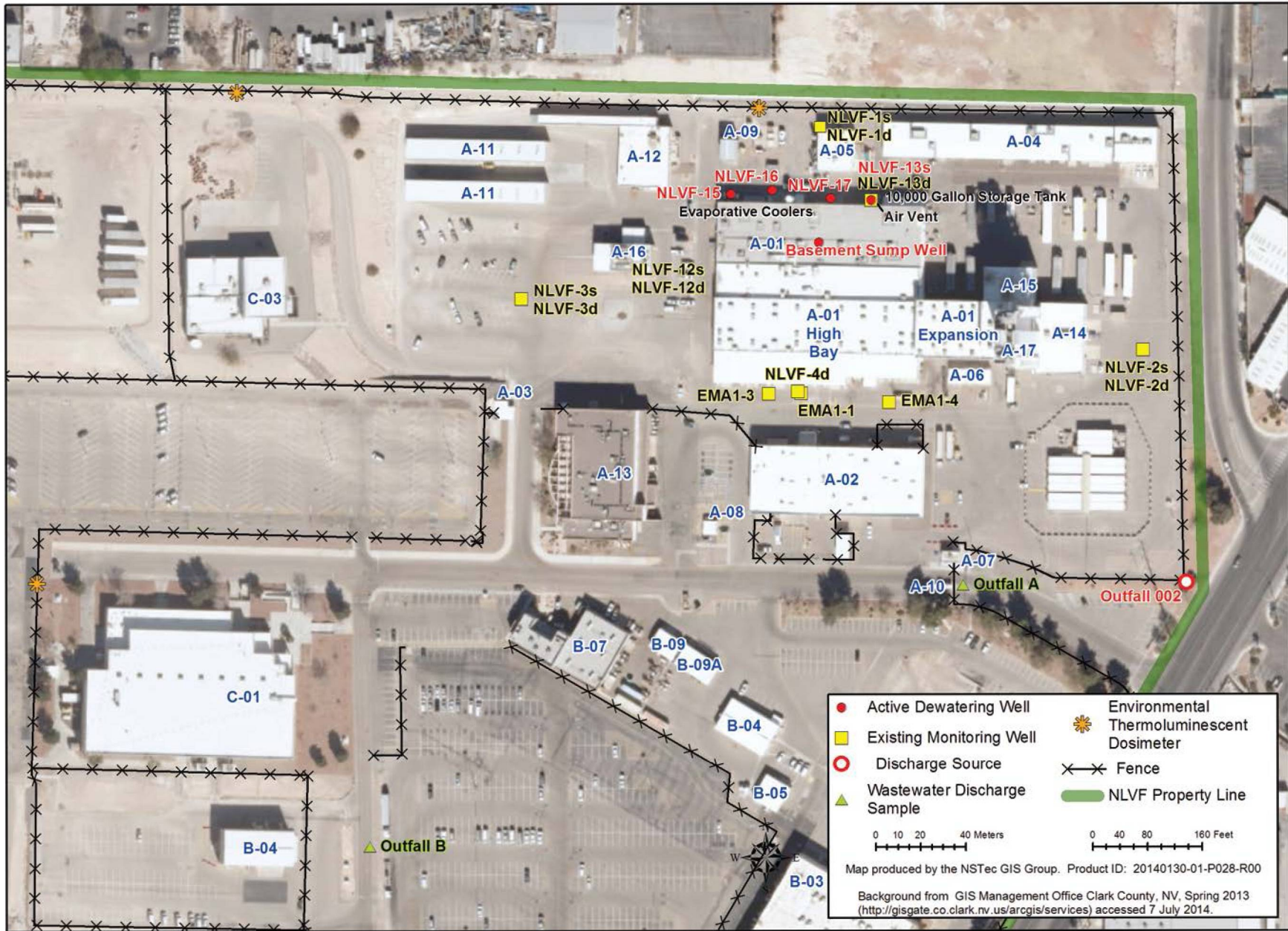
Figure A-2. Location of dewatering and monitoring wells around Building A-1
