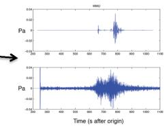
$$p(x, y, z; t) = \rho_0 \int_{S} \frac{\dot{u}(x', y'; t - \frac{R}{c_0})}{2\pi R} dS,$$
