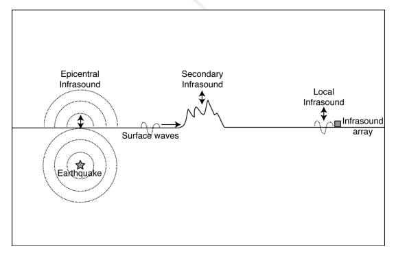
A schematic diagram illustrating different mechanisms of infrasound generation from earthquakes.
