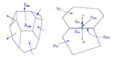
**Figure 3.1.** Space discretization and geometry data in the integral finite difference method (from *Pruess et al.* [1999]).
