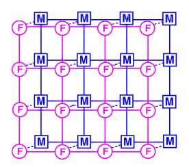
**Figure 2.9**. Flow connections in the "dual permeability" model. Global flow occurs between both fracture (F) and matrix (M) grid blocks. In addition there is F-M interporosity flow [*Pruess et al.*, 1999].
