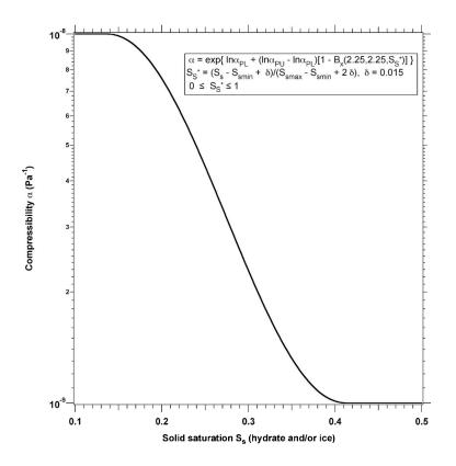
**Figure 2.5.** Compressibility of an unconsolidated porous medium impregnated with cementing solid phases (ice and/or hydrates). In this example,  $S_{Smin} = 0.15$ ,  $S_{Smax} = 0.4$ ,  $\alpha_{PU} = 10^{-8} \text{ Pa}^{-1}$ ,  $\alpha_{PL} = 10^{-9} \text{ Pa}^{-1}$  and  $\delta = 0.015$ .
