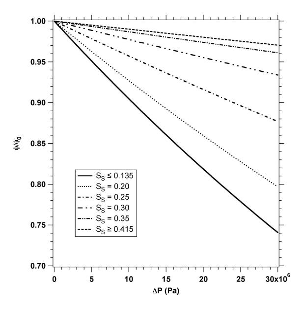
Figure 2.6. Effect of the varying compressibility described in Figure 2.5 on the porosity of an unconsolidated porous medium undergoing depressurization for various levels of saturation  $S_s$  of cementing solid phases.
