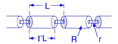
Figure 2.2. Tubes-in-series model of pore channels.
