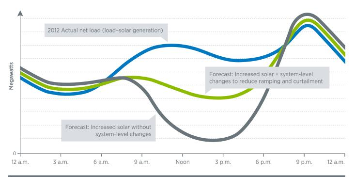
Figure 2. Without system-level changes, conventional generation must ramp more to accommodate increased solar generation.
