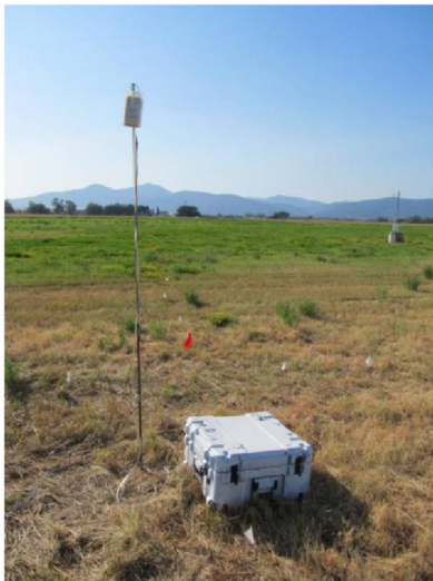
Figure 37 The Licor 820 sensor placed at the ZERT site. The inlet tube is at the top of the post to the left of the
