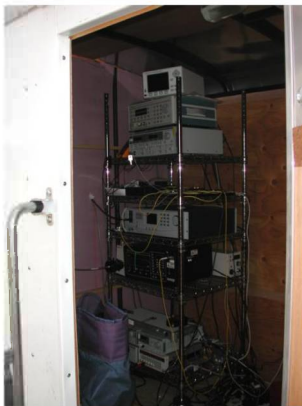
Figure 25 The electronics rack housed in the front of the trailer. A desk was also contained in this section for the instrument operator.
