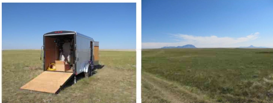
Figure 40 The left hand picture shows the DIAL instrument deployed in the cargo trailer at the BSCSP site while the right hand picture shows the view from the cargo trailer over which the DIAL was operated. The approximate site of the future production well will be approximately 1 km away from the where the trailer was located and would be in view of the left hand picture.
