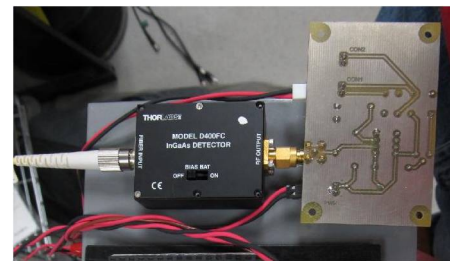
Figure 11 Photo of the seed laser check circuit attached to the optical detector.
