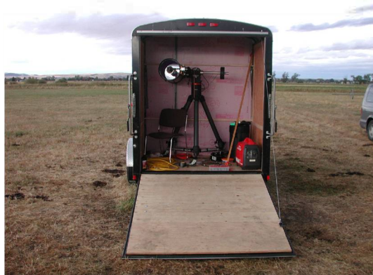
Figure 26 The scanning mount housing the output beam optics, telescope, and optical receiver train in the back of the trailer. The generator (seen in the lower right hand part of the trailer) was used to provide power to operate the instrument.
