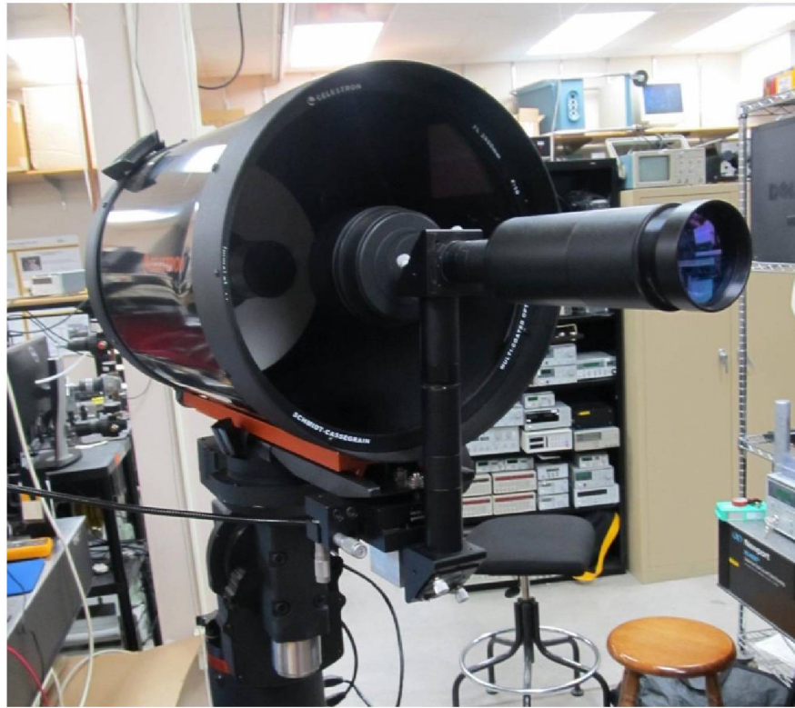
Figure 18 Another photo of the beam expander mounted to the telescope. The beam is entirely contained within SM1 optical tubing until it has been expanded to an eye-safe diameter of 5 cm.
