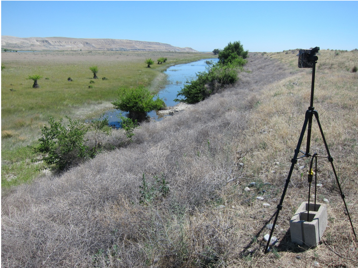
Figure 2. Field Camera Recording Surface Level Fluctuations at Pool 9 on the Hanford Site
