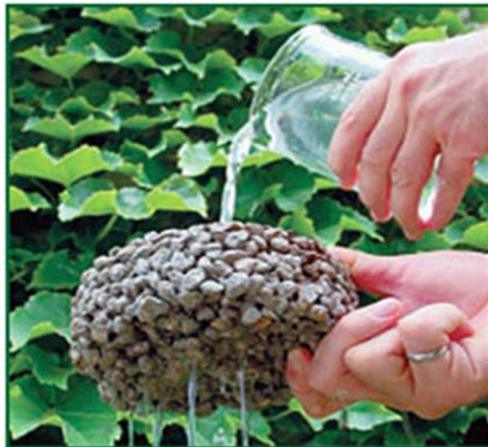
Figure 5. Example of water flow through pervious concrete (NRMCA).
