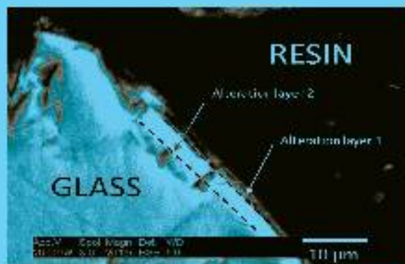
Figure 10. SEM picture performed in BSE of a granular SON 68 glass powder altered 9 months in 0.01 M \text{MgCl}_2 solution. Surface Volume = 40 \text{ cm}^2 .
