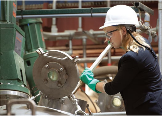
An NREL process engineer stirs a 1,450-liter fermentation vessel as part of biofuels research being conducted at the Integrated Biorefinery Research Facility. Photo by Dennis Schroeder, NREL 31690
