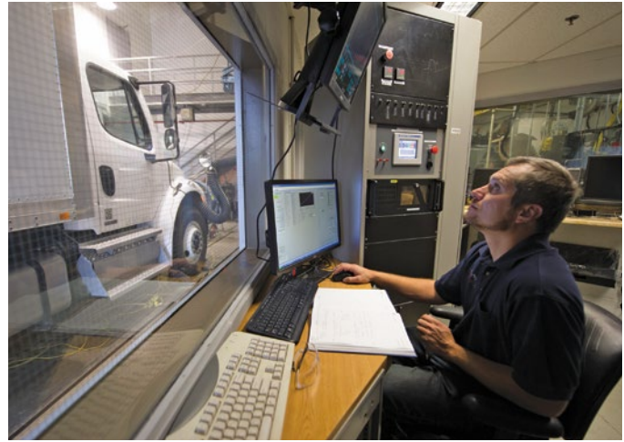
An NREL engineer monitors data from a test run on a chassis dynamometer in the control room at the Renewable Fuels and Lubricants Research Laboratory. Photo by Dennis Schroeder, NREL 22761
