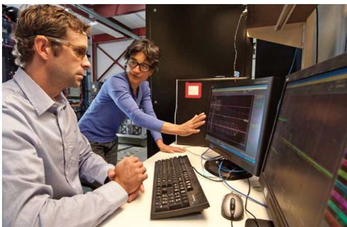
NREL researchers analyze micro-grid synchronization wave forms at the NWTC's Distributed Energy Resources Test Facility to facilitate interconnection and grid integration of renewable energy sources. Photo by Dennis Schroeder, NREL 21937
