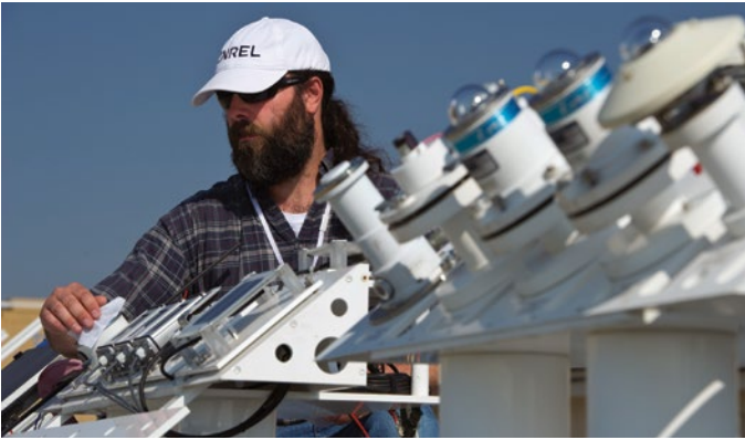
An NREL researcher cleans individual photovoltaic cells at the Outdoor Test Facility to measure the variance in performance between an uncleaned cell and a cell cleaned daily of dirt and pollutants. Photo by Dennis Schroeder, NREL 21326
