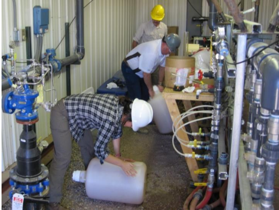
Figure A-5. Mixing concentrated tracer solutions in carboys.
