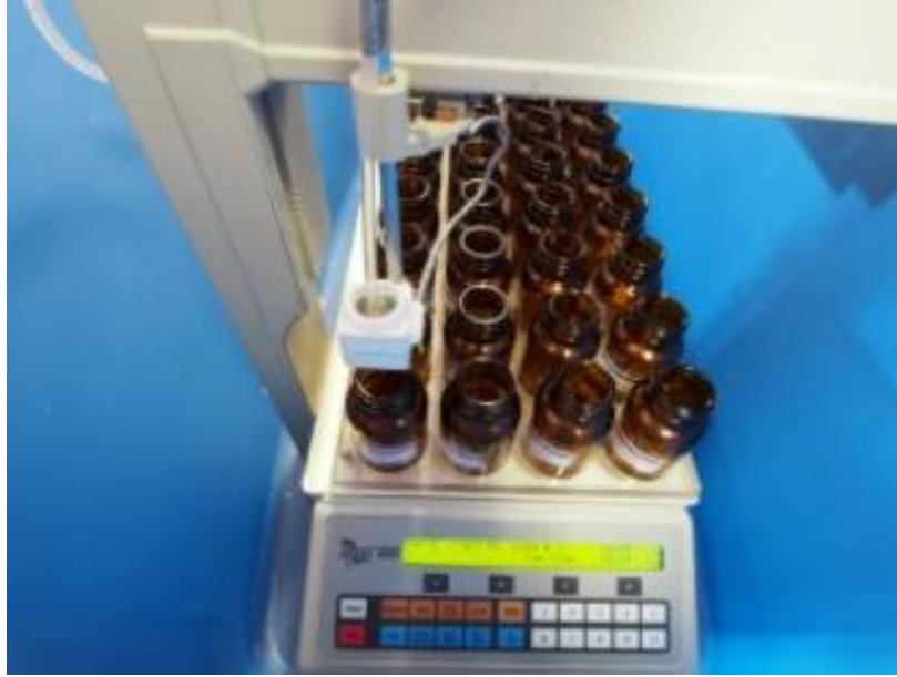
Figure A-7. Close-up view of autosampler loaded with sample bottles inside bin.
