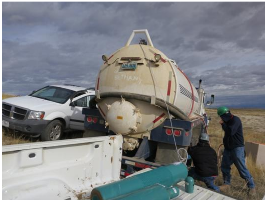
Figure B-4. Purging tank truck headspace with CO 2 /H 2 /N 2 gas mixture at MP-423.
