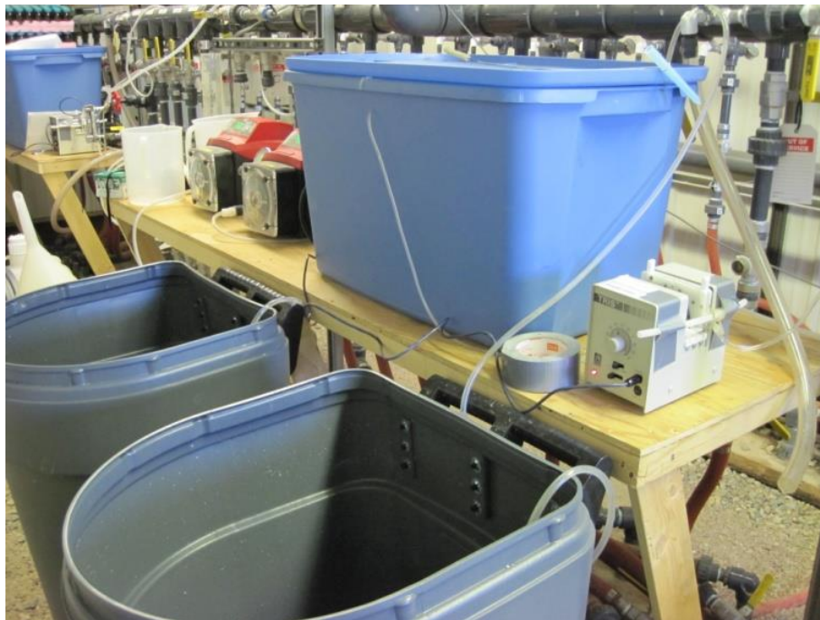
Figure A-6. Garbage bins used for dispensing concentrated tracer solution, and high-pressure peristaltic pumps (red) used to inject tracer into circulating injection flows. Autosampler is inside of blue bin on shelf; peristaltic pump feeding autosampler is to right of bin.
