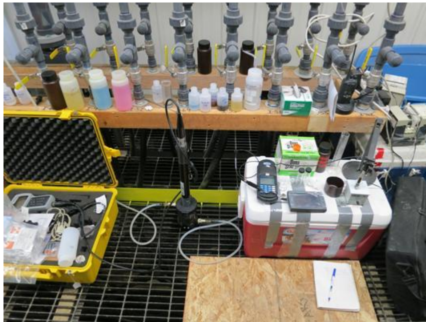
Figure B-6. YSI sonde and meter with flow cell inside HH 7-5. Cooler top was used for alkalinity measurements and Hach reagent kit measurements of \text{Fe}^{2+} and \text{S}^{2-} .
