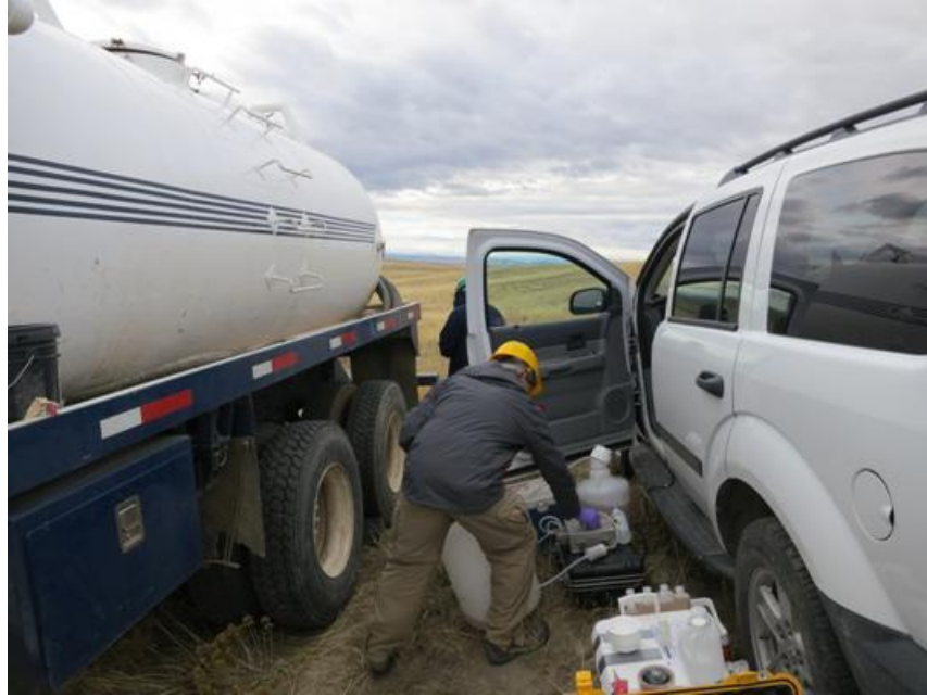
Figure B-3. Measuring field parameters with YSI sonde/meter and Hach kits while tank truck is being filled with 4P-61 water.
