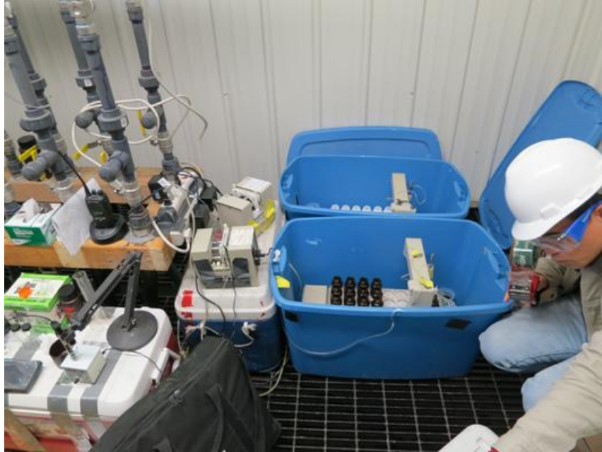
Figure B-7. Dual autosampler setup in HH 7-5 to collect samples for tracer analyses and also for uranium and general chemistry analyses.
