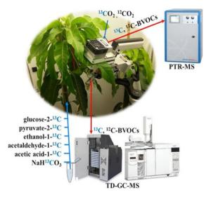
Figure 2. Experimental setup for Geco leaf-level study.
