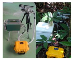
Figure 3. Portable photosynthesis and VOC emission system.
