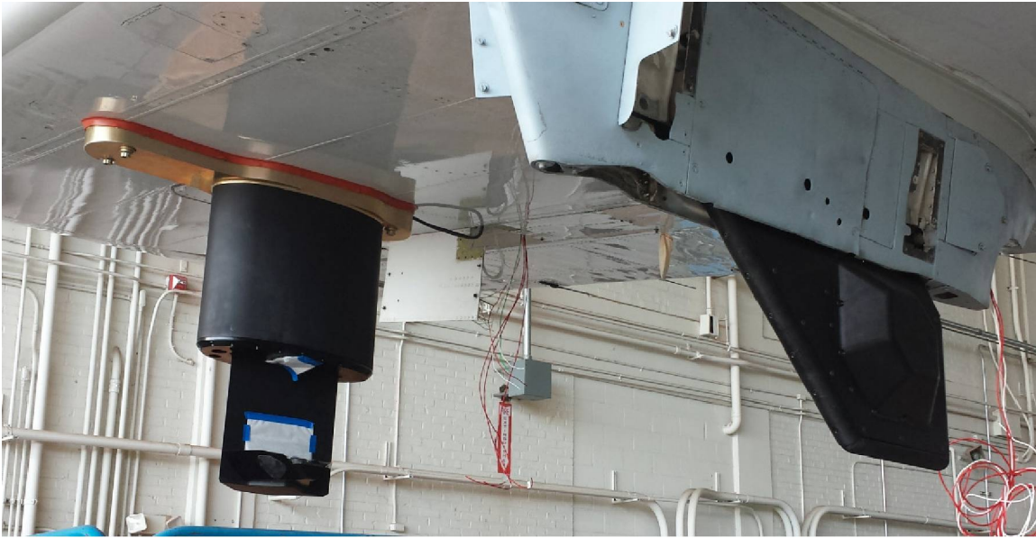
Figure 7. TO-I-Neph fully integrated beneath the wing of the NASA P-3.
