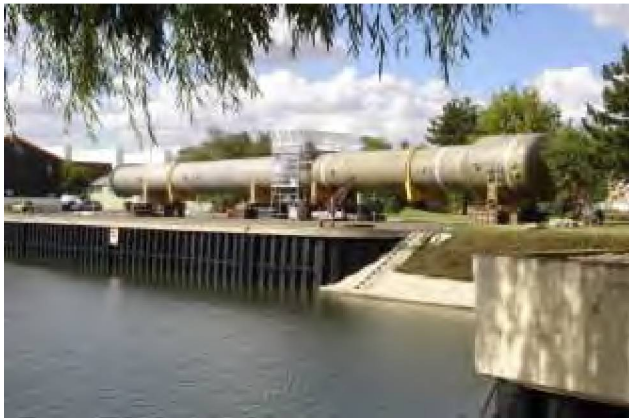
Figure 3-39: Example of Cryogenic Distillation Column Before Transportation
