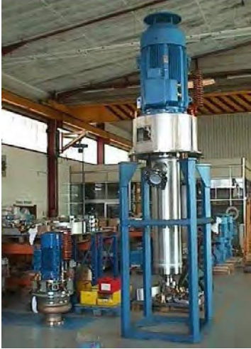
Figure 3-35: Typical Cryogenic Centrifugal Pump
