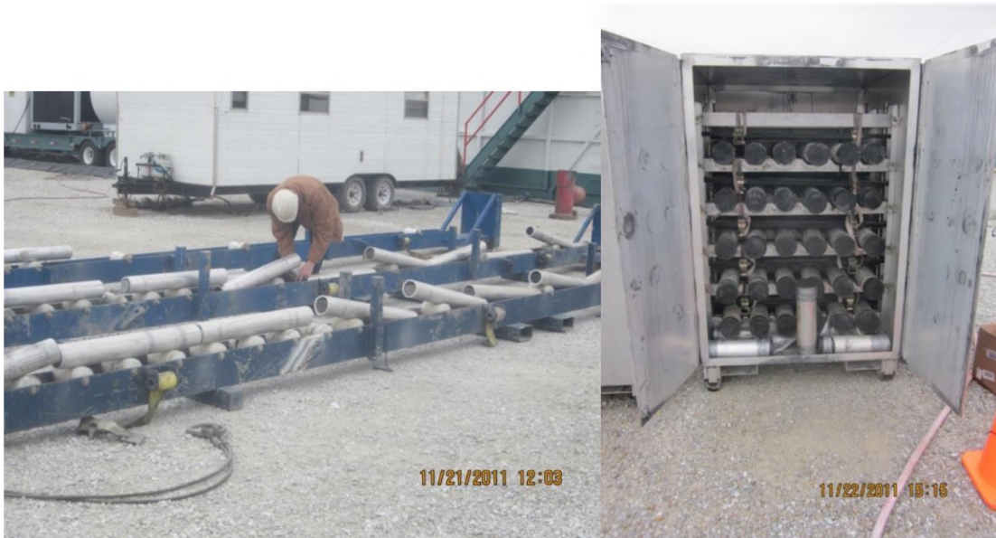
Figure 4.28. Cutting Core into Sections for Shipment to the Core Analysis Laboratory (left) and the Shipping Container (right)
