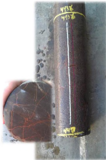
Figure 4.69. Precambrian Meta-Rhyolite from Stratigraphic Borehole FGA-1. Longitudinal and end view of full diameter core. End view shows altered surfaces along fractures.
