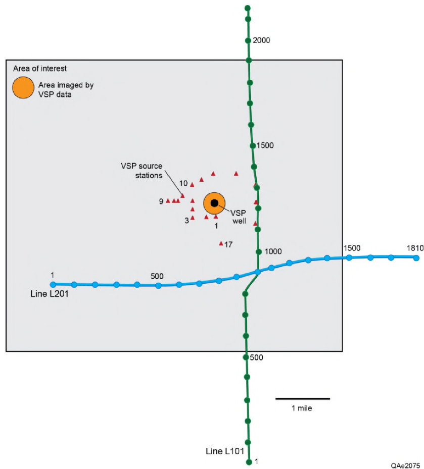
Figure 4.46. Location of Borehole VSP (Stratigraphic Borehole FGA-1) and Surface Seismic Data Acquired at the FutureGen 2.0 CO 2 Storage Site
