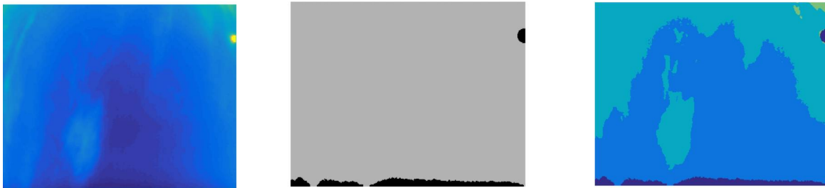
Figure 2. ICI images from Barrow: radiance in W\ m^{-2}\ sr^{-1} (left), conventional binary cloud map showing cloudy and clear pixels (center), and cloud map showing upper-limit cloud optical depth (right).
