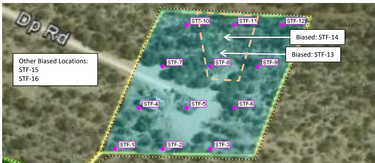
Figure A2. Map of sampling locations in the STF decision area for tract A-16-d. Grid locations are indicated with pink dots. Biased locations are indicated for STF-13 and STF-14 in the dash-outlined outfall area. Two additional biased locations should be field-located within the dash-outlined area. Note: Map locations and boundaries are approximate.
