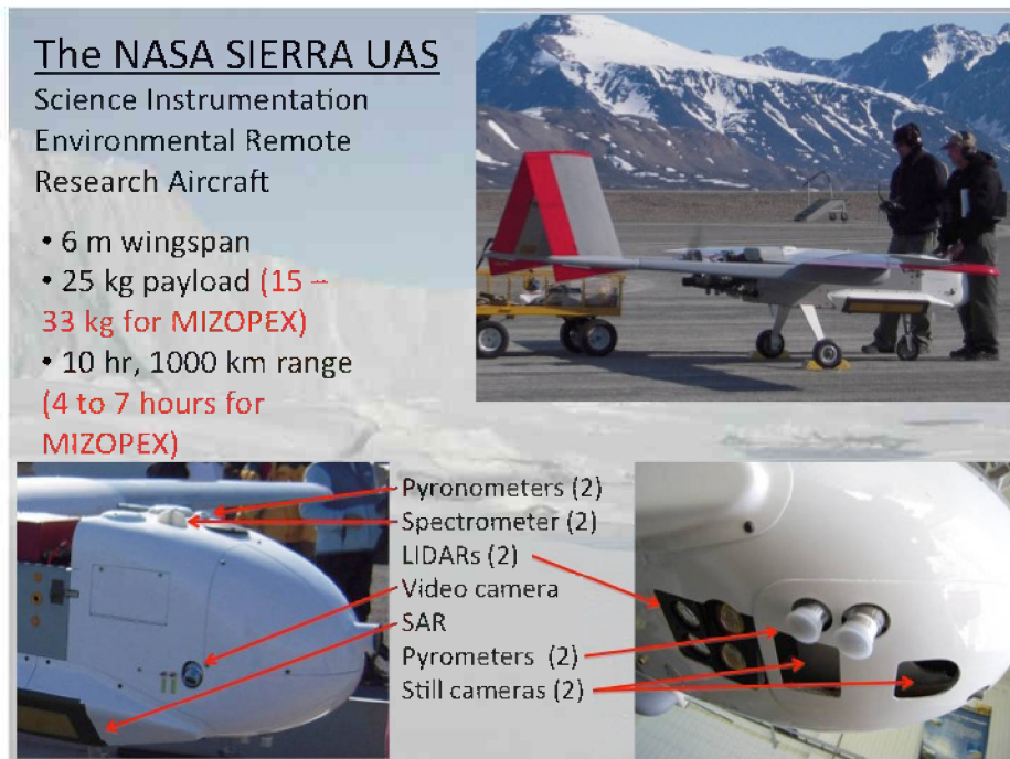
Figure 6. Overview of the NASA SIERRA UAS as configured for Svalbard operations during the Characterization of Arctic Sea Ice Experiment (CASIE).
