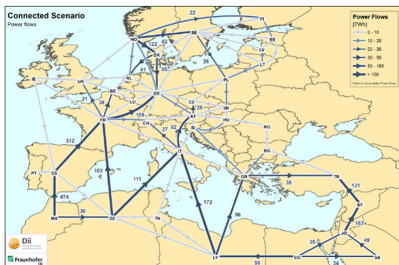
Fig. 12 - Connected DESERTEC 2050 scenario power flows. Source: Zickfeld and Wieland 2012
