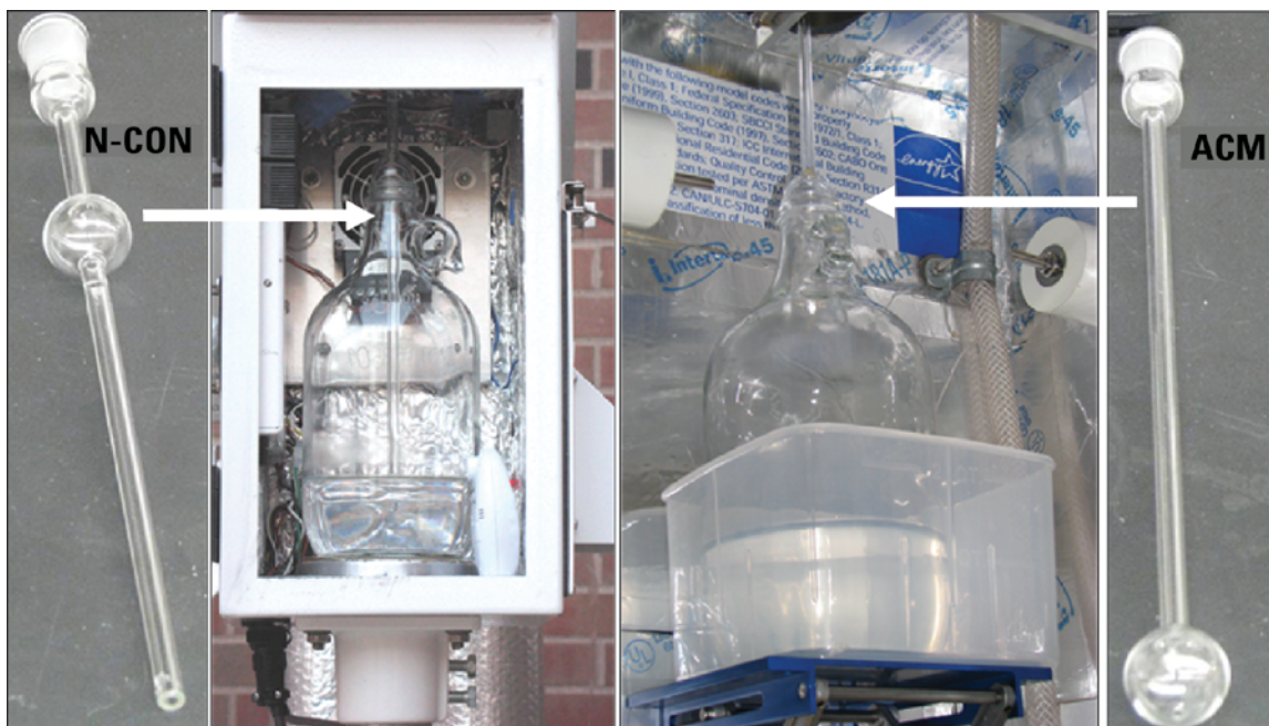
Figure 18. Thistle-tube configurations used with the modified N-CON collector (left) and the ACM collector (right).
