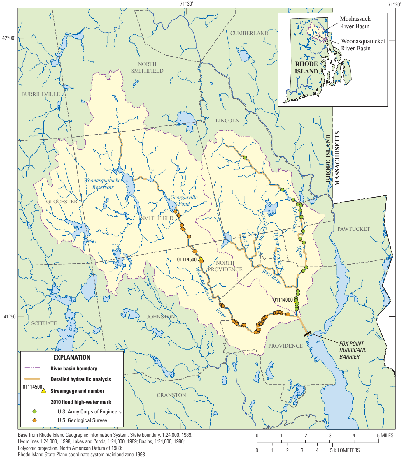
Figure 2. High-water marks obtained after the 2010 flood along reaches of detailed hydraulic analysis in the Moshassuck and Woonasquatucket Rivers, Rhode Island.
