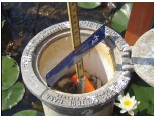
Figure 5. An elevation benchmark (left) and measurement of water-level elevation (right). From Volin and others (2008).
