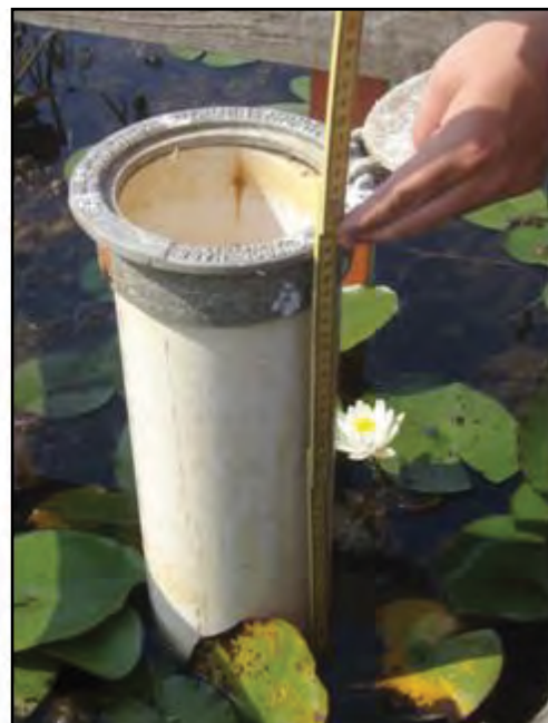
Figure 5. An elevation benchmark (left) and measurement of water-level elevation (right). From Volin and others (2008).
