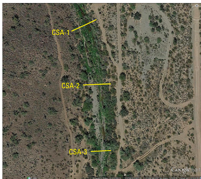
Figure 20. Aerial view of the Deadman Wash near New River, Arizona, continuous slope-area (CSA) reach. Cross sections are shown in yellow. Flow is from top to bottom. Image is from Google Earth and was taken March 15, 2015.
