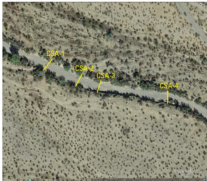
Figure 25. Aerial view of the Delaney Wash, Arizona, continuous slope-area (CSA) reach. The cross sections are shown in yellow. Flow is from left to right. Image is from Google Earth and was taken December 29, 2014.
