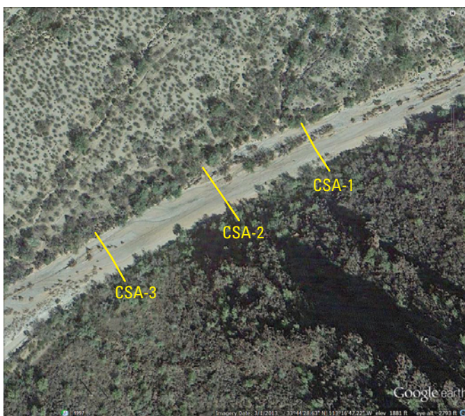
Figure 41. Aerial view of the Tiger Wash near Aguila, Arizona, continuous slope-area (CSA) reach. Cross sections are shown in yellow. Flow is from right to left. Image is from Google Earth and was taken March 1, 2013.
