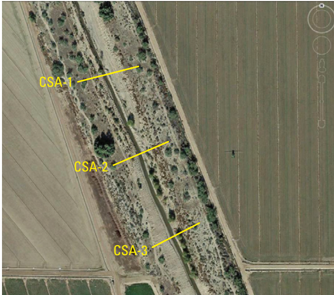
Figure 28. Aerial view of the Hassayampa River near Arlington, Arizona, continuous slope-area (CSA) reach. Cross sections are shown in yellow. Flow is from upper left to lower right. Image is from Google Earth and was taken December 29, 2014.
