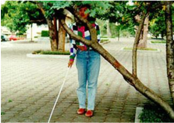
Figure 33: Overhanging tree hazard for blind people. Photo: Japanese Society for Rehabilitation of Persons with Disabilities
