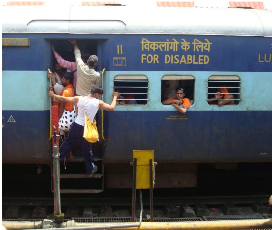
Figure 57: Train car for "Disabled" that is not accessible. Photo: Svayam/Jindal Saw Ltd.
