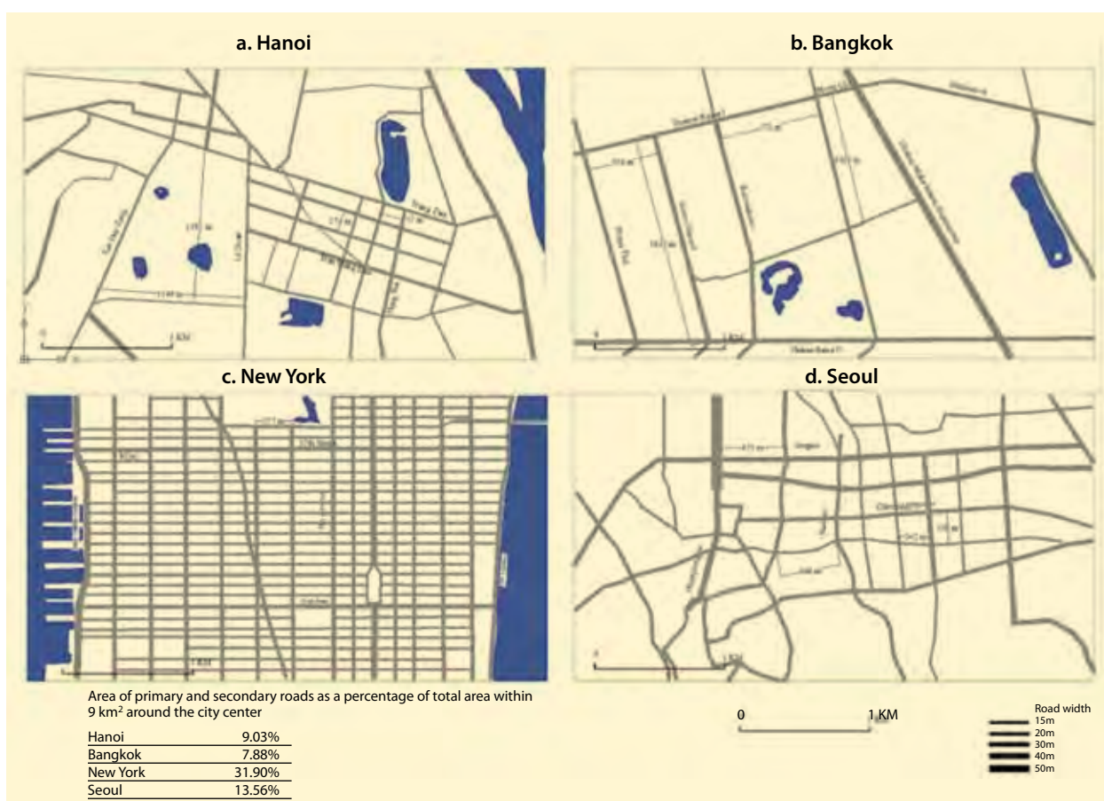
MAP 2.2 Street densities compared: The central business districts of Bangkok, Hanoi, New York, and Seoul
