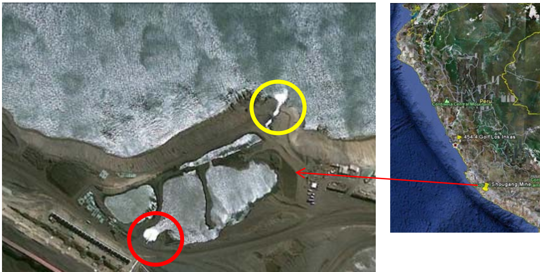
Figure 3. Water flow into a settlement lagoon (red circle) at an iron ore concentration facility on San Nicolas Bay (Marcona, Peru) and the discharge into the sea (yellow circle). The area shows a high species diversity and is close to two marine protected areas with colonies of sea lions and penguins.
