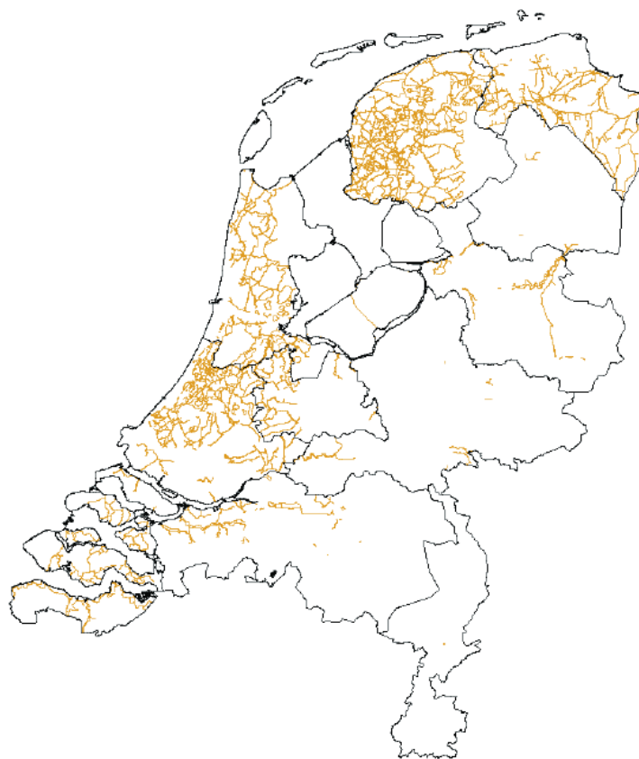
Figure 36: (In yellow) secondary flood defense system, 15 000 km, the safety standards have been set by the provinces [Inspectie Water 2011], Provincial boundaries are given in black.
