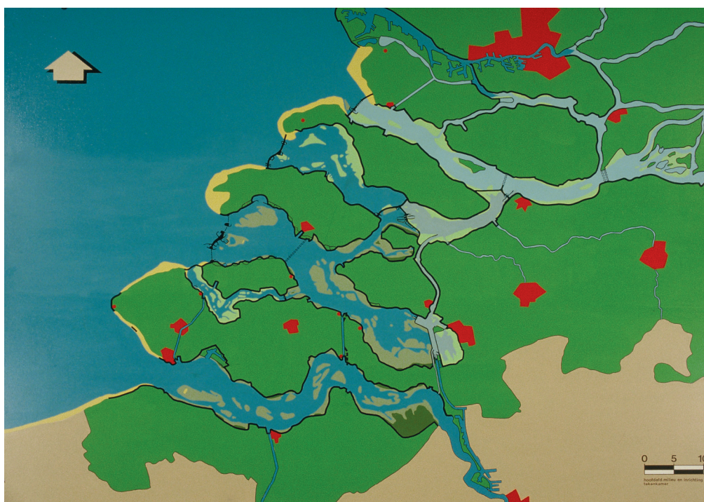
Figure 6: The delta plan consisted of 4 main barriers and 6 secondary barriers in the Rhine, Meuse and Scheldt Estuaries.
