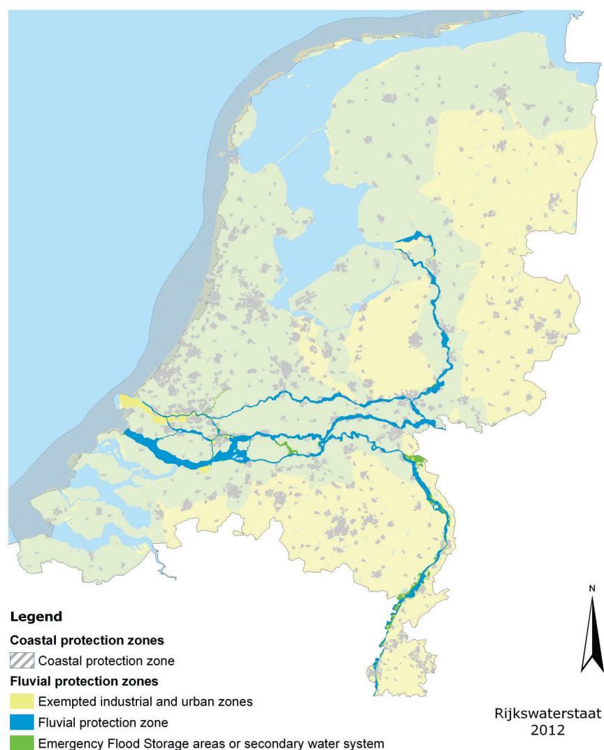
Figure 34: Zones with specific rules for rivers, the flood plain and the dune coast regarding flood defenses.
