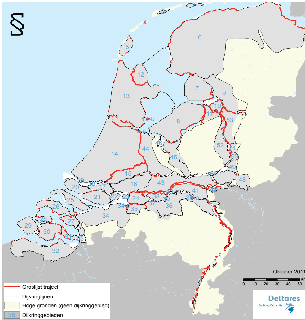
Figure 50: Flood Defenses in need of repair or with ongoing repair
