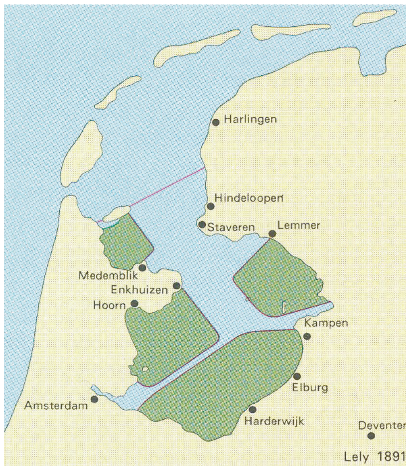
Figure 41: The Zuiderzee project in 1891 by Engineer Lely, [Duin, R.H.A. van and Kaste, G. de, 1990]
