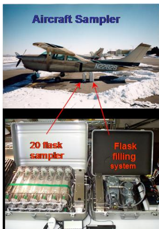
Figure 1: NOAA installation for sampling vertical profiles.
