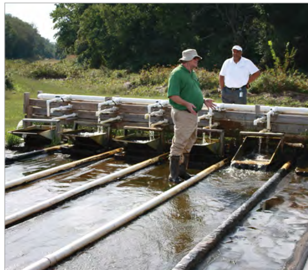
New BMPs may be considered for inclusion in a trading program through an approval process, which can be more or less formal. Photo of algal mats treating ditch water courtesy of American Farmland Trust.
