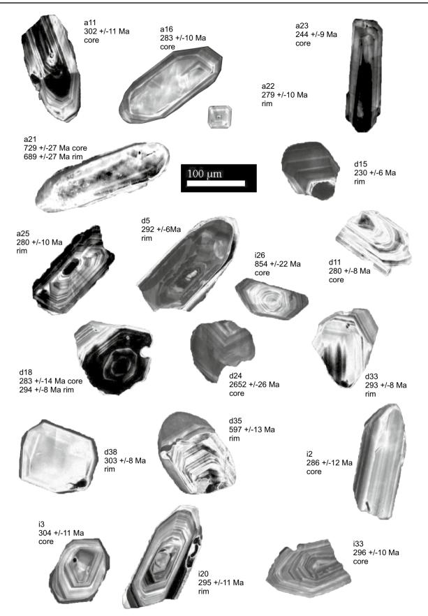
Fig. 14 Representative cathodoluminescence (CL) images of analyzed zircons separated from the felsic layer of the uppermost Rogdia Beds (Q6 subunit); sample 24-09-07/1-3
