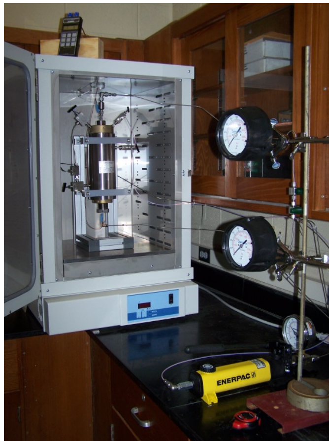
Figure 1.1.5. Triaxial core holder in an oven, for measurements using supercritical CO 2 .
