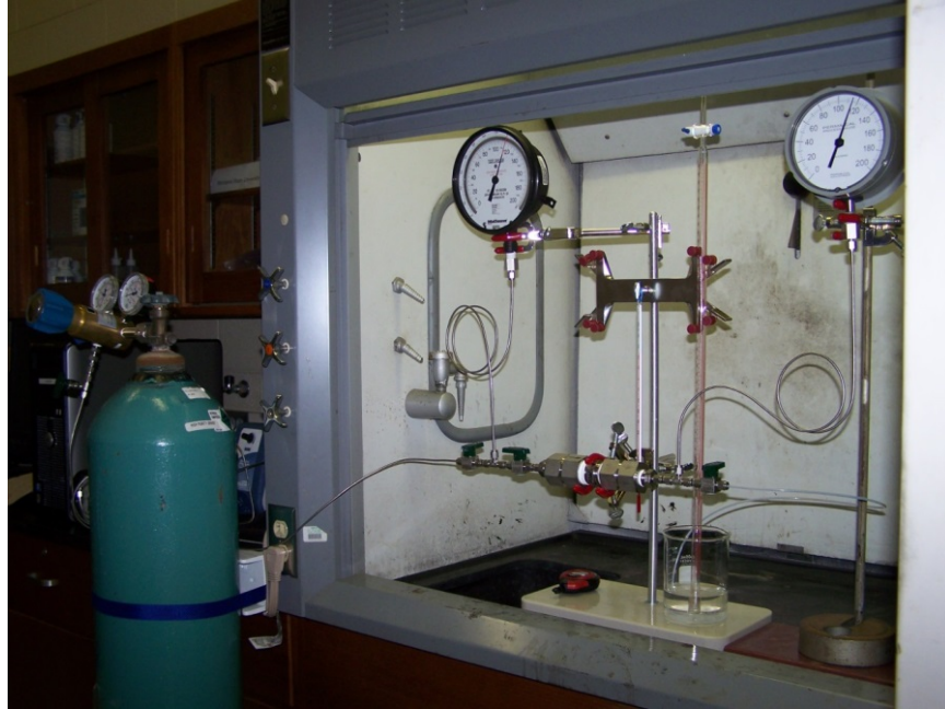
Figure 1.1.3. Early setup for measurement of permeability by steady flow. The sample cell shown in Figure 1.1.2 is in the lab clamp below and to the right of center in this photo. The flow rate of nitrogen gas through the core plug was measured by timing the displacement of water from the inverted burette or a graduated cylinder at higher gas flow rates. Slight reconfiguration of the plumbing enabled measurements by pressure-pulse decay.
