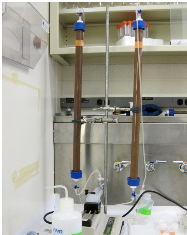
Figure 2. Photo of columns used for the column transport experiments.
