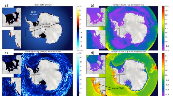
Snapshot from year 6 of a sample simulation showing ice melt rate due to interaction with the ocean, ocean surface temperature, ocean surface current speed, and ocean bottom temperature. Lower right shows the invasion of relatively warm water onto the continental shelf that can rapidly melt the Pine Island Glacier.
