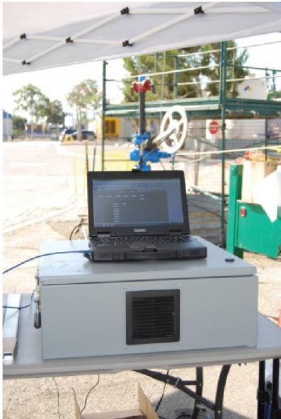
Figure 58 SUS-CO 2 -DICAST system during field validation, and sensor signal during first detection of CO 2 in the field at 1,000 ft. and 251 psi.
