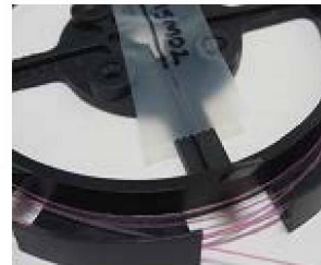
Figure 8 Sensor materials coated on glass slides for preliminary evaluation and fiber optic sensor prototypes fabricated with the selected formulations.
