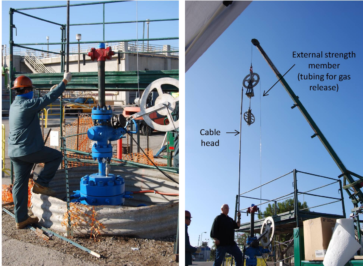
Figure 54 (left) 5,200 ft. well head. (right) First step of the deployment, introducing the cable head into the well.
