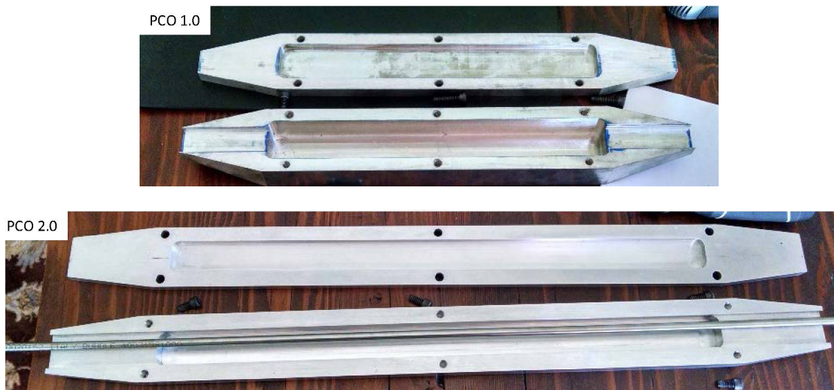
Figure 53 First version (PCO 1.0) and revised version (PCO-2.0) of the connector protector.
