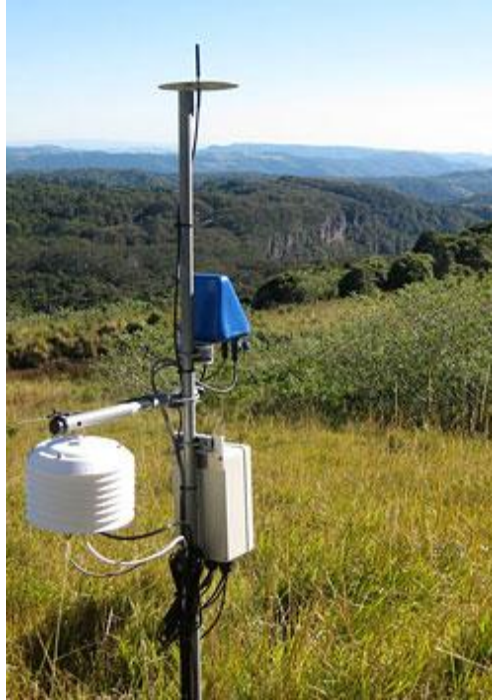
Figure3-5: Springbrook Wireless Sensor Networks
